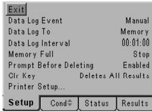
The Model 4520 has a variety of options relating to the storage of data. To initiate data logging the Data Log Event setting should be ENABLED. By default this option is MANUAL.
