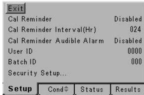
A reminder that calibration is due can be set via the Cal Reminder option. Once this option is set a valid calibration is required to use the 4520 after the time limit has elapsed. This option is DISABLED by default.
