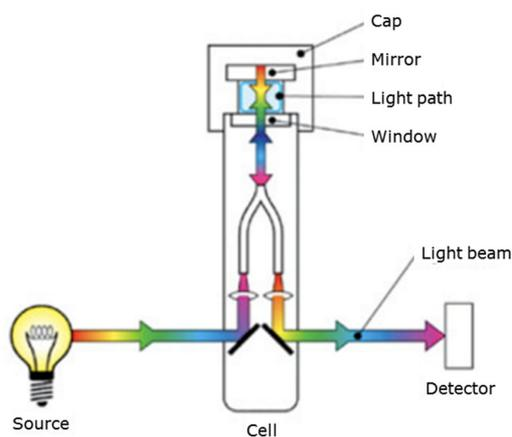
The TrayCell is first positioned in the cell holder of the spectrophotometer and a droplet of sample is placed on an optical window on top the surface of the cell. A cap containing a mirror is then fitted over the top. The type of cap used determines the path length through which the light passes.
