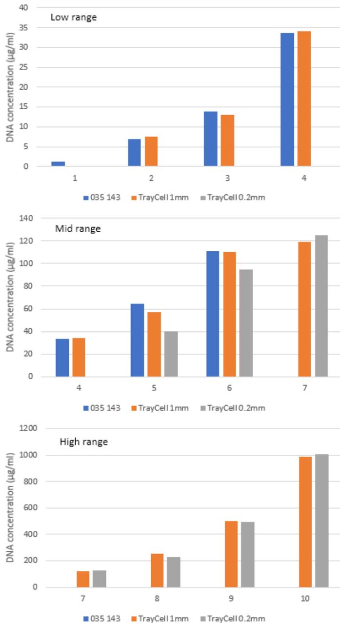
The results demonstrate that the TrayCell gives comparable values to the samples measured in conventional 10mm path length cuvettes up to the limit of the spectrophotometer absorbance range. The results also clearly show that due to the virtual dilution factor of the TrayCell caps, it is possible to measure DNA of a much higher concentration (greater than 125µg/ml) than standard cuvettes avoiding dilution of the sample.
